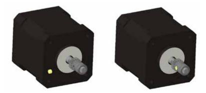
**2.** Lock the head screw of M3\*2 and prefix the extrusion wheel.
