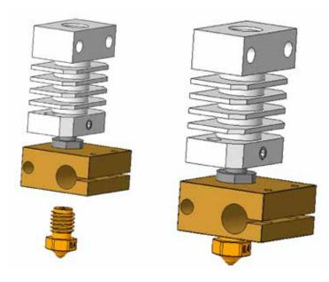
**3.** Screw the nozzle into the heatblock.
