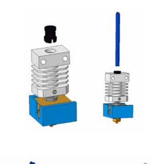
**7.** Install bowden collect on the hotend and the Teflon tube.
