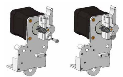
**5.** Lock step screws. Adjust the relative position of the active extrusion wheel on the motor and the driven extrusion wheel on the swing arm to make the front and rear positions consistent, then lock the head screw of the active extrusion wheel on the motor (M3\*2).
