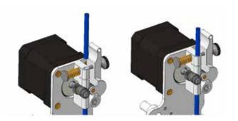
**11.** Insert Teflon tube into the upper end of the backplane (self-provided).
