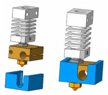
**4.** Install the silicone sock. (Before this step, you could install heating rods and thermistors first).
