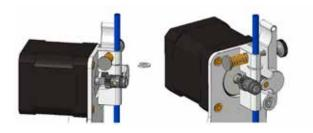
**12.** Insert the E-type spring into the cut on the backplane to fix the Teflon tube.
