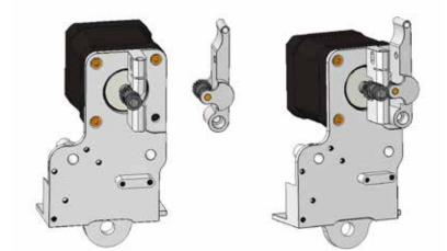
**4.** Align the countersunk holes on the swing arm with the four holes of the motor.
