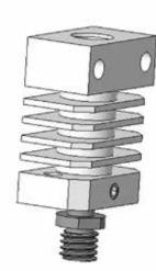
**1.** Install the heatbreak on the heatsink and lock the head screw.
