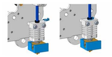
**10.** Adjust the direction of the Teflon tube so that the cut at the place of the extrusion wheel is consistent with the backplane.
