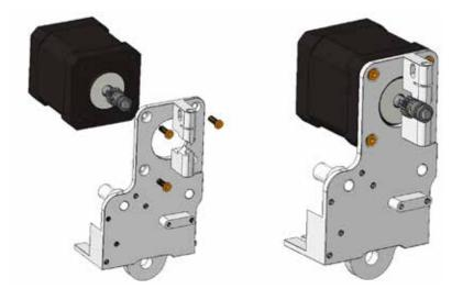
**3.** Lock the motor into the backplane through three countersunk screws.
